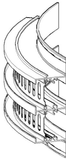
LINEAR SLOT CURVE INSIDE WALL
